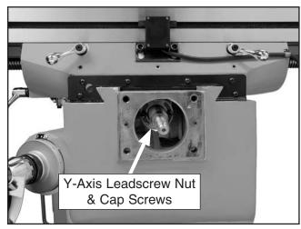
Figure 68. Y-axis leadscrew nut and cap screws.
